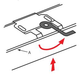
Push the swing arm clockwise to lock firmly while holding the headrail fixedly.
