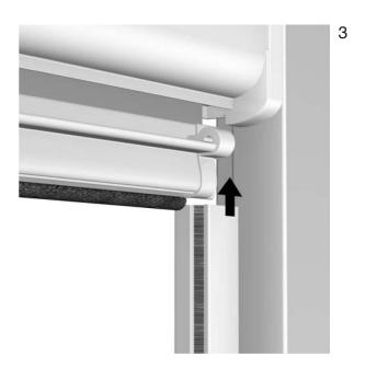
Fix the side tracks as per picture. Use a screw driver narrow enough to allow you to screw all the way in the track, the head of the screw must be flat with the back of the track.
