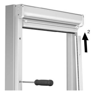
Remove all the plastic covers on the side tracks to expose hole.
